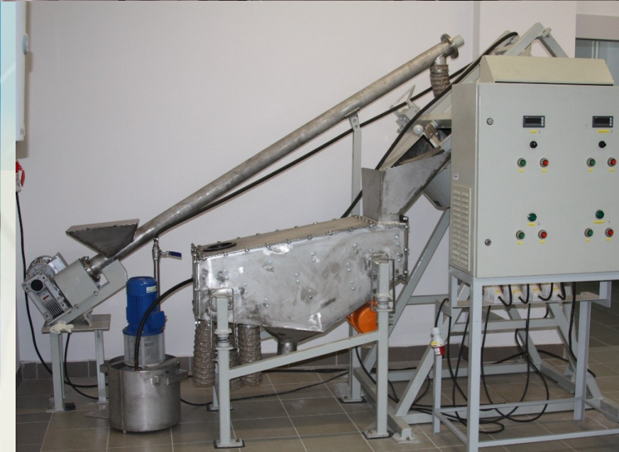
Figure 6. Large scale granulator for waste based fertilizers production (disk diameter = 80 cm)
